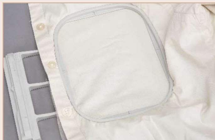
Fig. 4-6. Tightening the hoop too much causes ripples in the hooped fabric.
