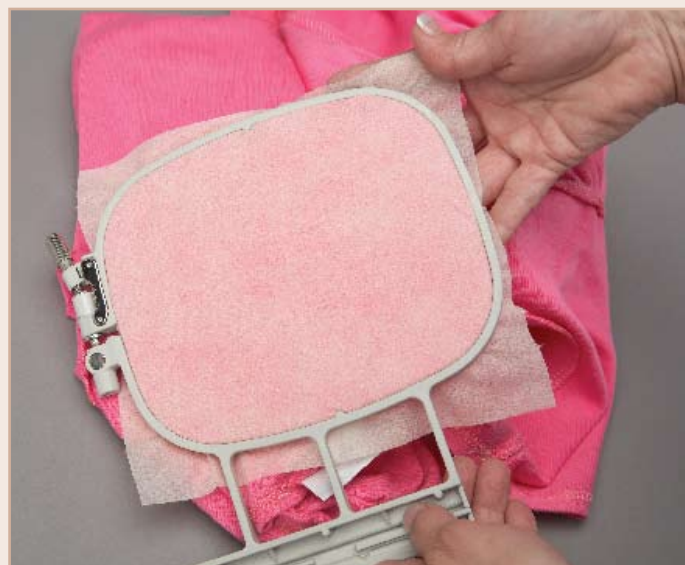
Fig. 4-7. Don't skimp on the size of your stabilizer. It should extend from all hoop edges.
