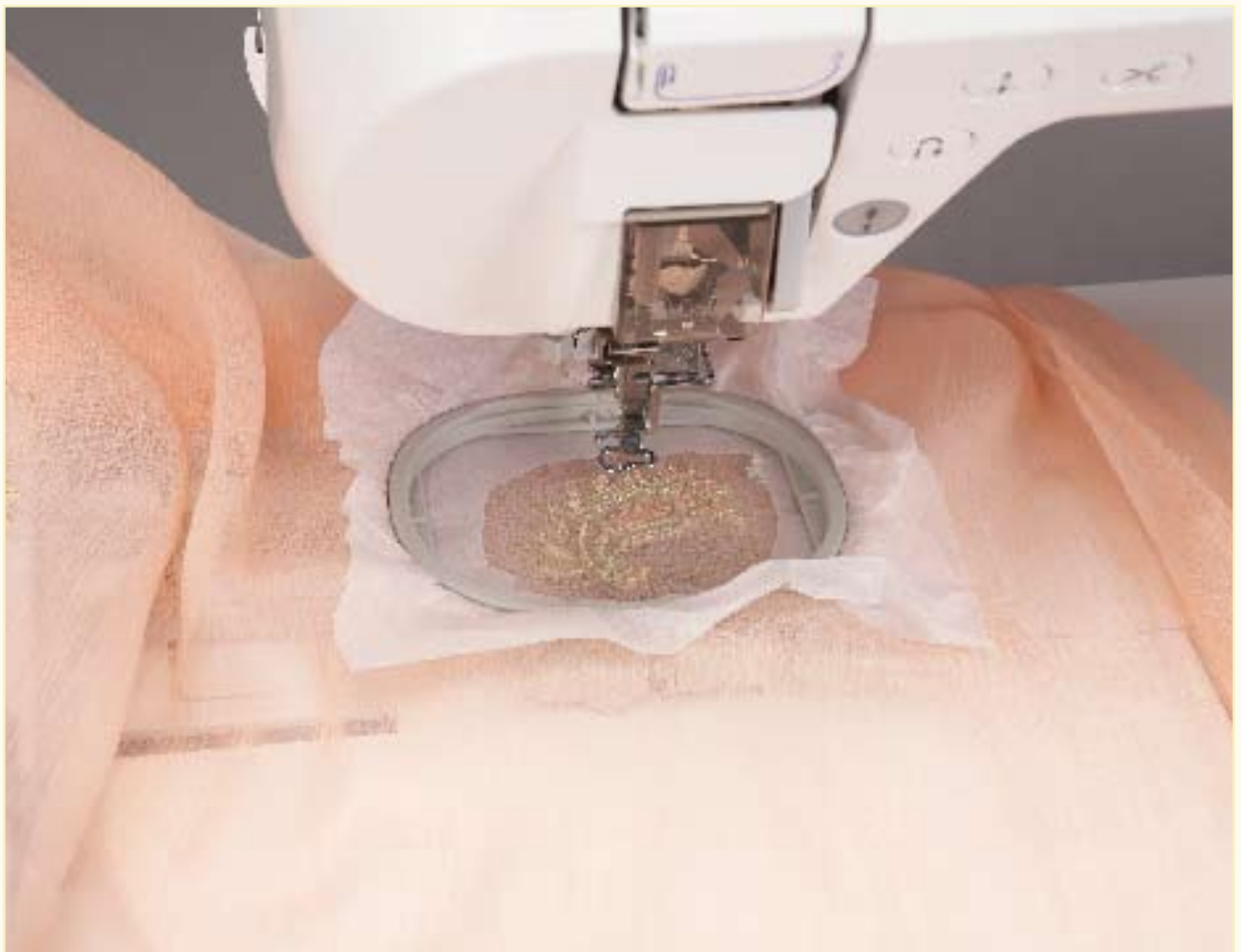
Fig. 9-4. A simple buffer of tissue, matte side facing fabric provides grip and avoids marring of delicate sheer fabrics.
